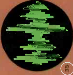
35 MUSICAL TONE, WITH VIBRATION PICK-UP APPLIED TO MUSICAL INSTRUMENT.
