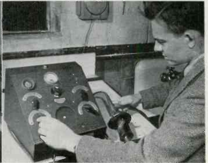
ELECTRONIC coil tester in Cities Service laboratory
