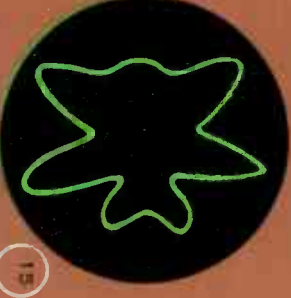
14 OUTPUT FROM CLIPPER AMPLIFIER IN A TYPE OF WAVE SHAPING CIRCUIT.
