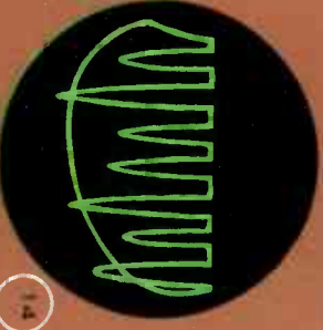
13 AN AUDIO-FREQUENCY TONE WITH STRONG 15th HARMONIC OR OVERTONE SUPERPOSED.
