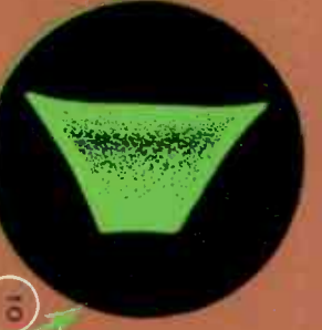
10 MODULATED R.F. SIGNAL, USING AUDIO MODULATING TONE AS THE TIME BASE.
