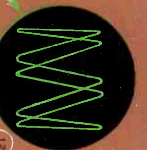
12 LISSAJOU FIGURE, TWO SINE WAVES APPLIED TO DEFLECTION PLATES WITH 5:1 RATIO.
