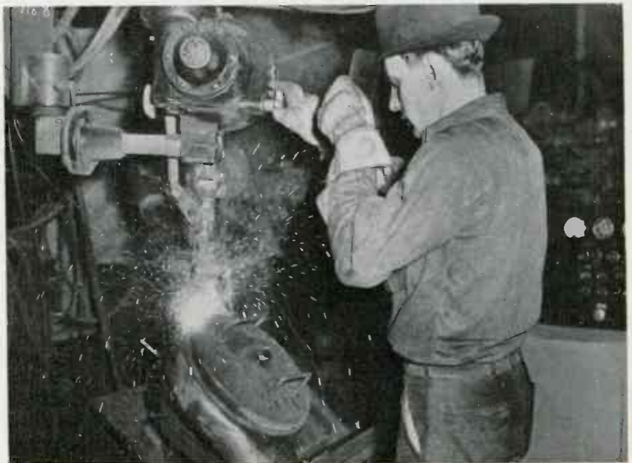
MOTOR CONTROL , applied to arc-welding equipment used in fabrication of automotive axle-housings. Electrode is fed at pre-set rate
