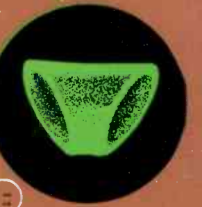
11 SIMILAR TO 10 (at left) BUT WITH A PHASE SHIFT SHOWING IN AUDIO SYSTEM.
