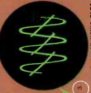
3 DOUBLE TRACE USING ELECTRONIC SWITCH, SINE & SAWTOOTH WAVES COMPARED.
