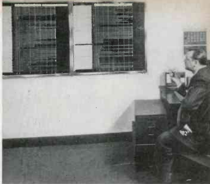
GLANCE SHOWS SITUATION in production and materials programs at Emerson Radio plant in New York. Production board made by Wassell Organization, Westport, Conn., here gives due-dates of all materials, shows which are behind schedule and which are coming in on time
