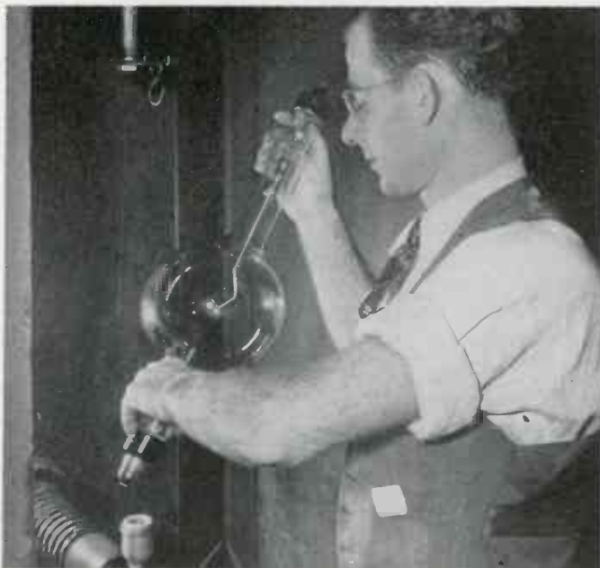
SAFETY FOR X-RAY WORKERS is provided by bit of film clipped to vest. Developed each week, film reveals whether worker is receiving dangerous amount of radiation. Idea comes from Westinghouse X-ray tube test department
