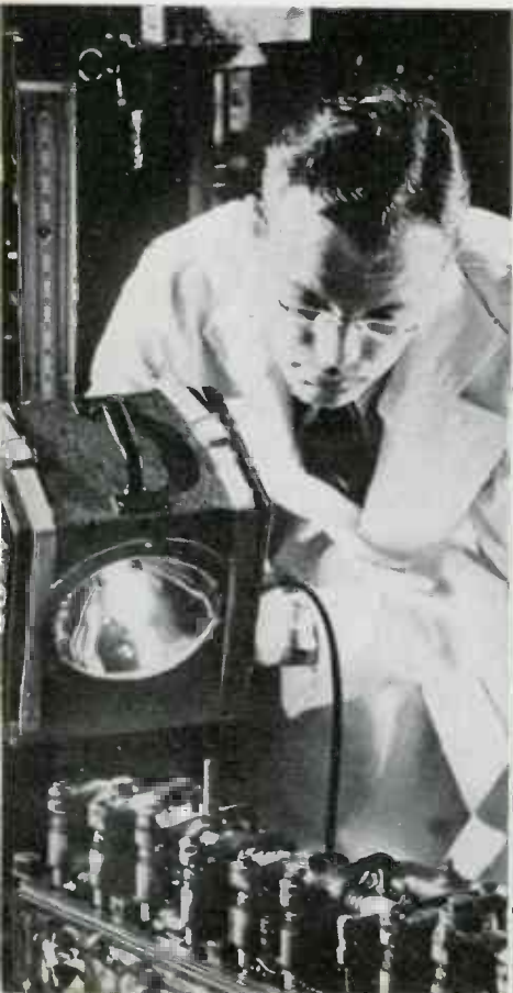
ROCKER-ARM action under "slow motion" study with Gen'l Radio Strobolux
