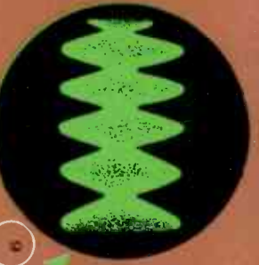
9 MODULATED R.F. SIGNAL, USING LINEAR TIME BASE IN THE OSCILLOGRAPH.
