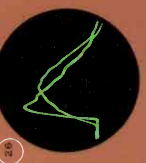
29 SQUARE WAVE CHECKED WITH INTERRUPTED TRACE, TIMED BY "Z" AXIS CONTROL.
