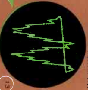
13 AN AUDIO-FREQUENCY TONE WITH STRONG 15th HARMONIC OR OVERTONE SUPERPOSED.
