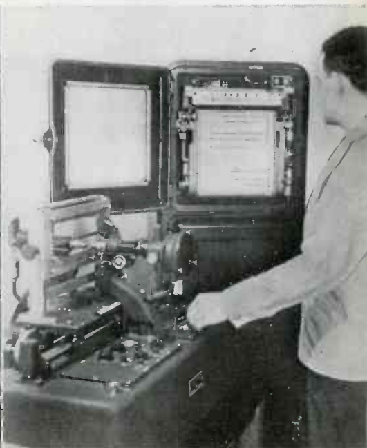
SPECTROGRAPHIC analysis is simplified by automatic equipment for scanning and recording densities of spectrogram lines of unknown material. Unit shown made by Leeds & Northrup, Philadelphia, Pa.
