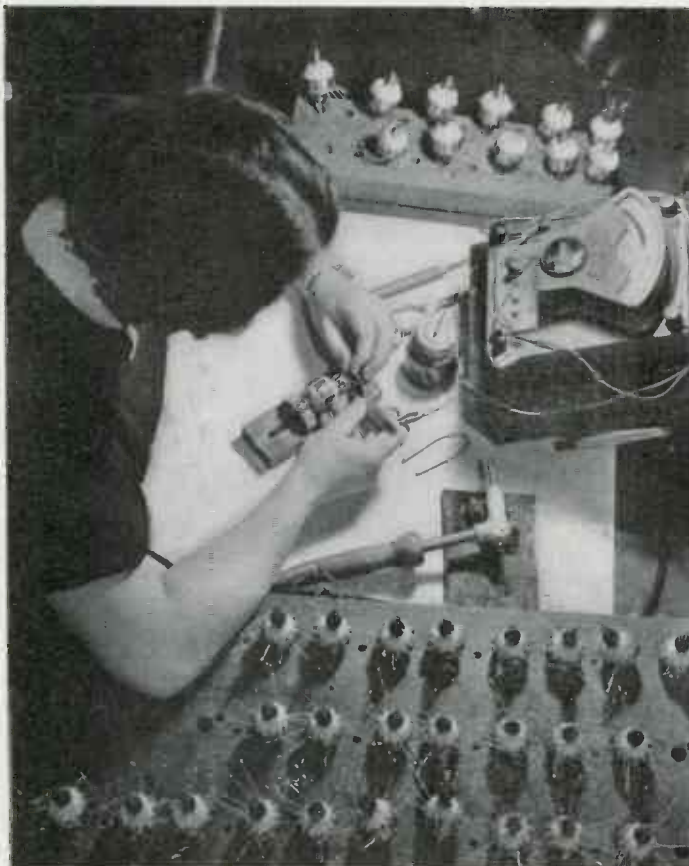
SPECIAL SOLDERING IRONS made to fit a particular job often speed work. Right-angle iron shown in use at Weston, Newark, N. J., plant
