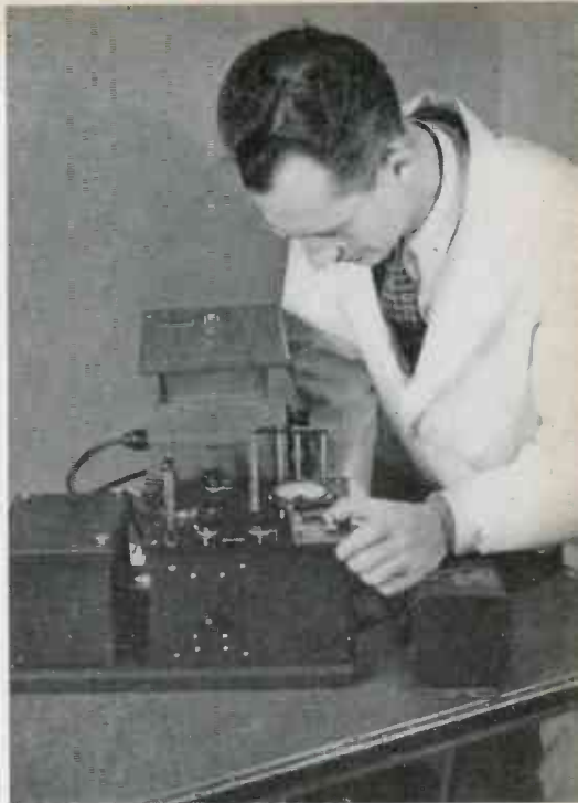
CHEMICAL COLORIMETER and → color grader made for Hercules Powder Co., Wilmington, Del., by Rubicon Co., Philadelphia. Single meter reading gives resin sample's ratio of transmission for light beams of two different colors
