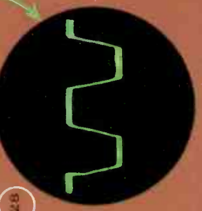
26 SQUARE WAVE CHECKED WITH INTERRUPTED TRACE, TIMED BY "Z" AXIS CONTROL.
