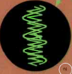
2 DOUBLE TRACE USING ELECTRONIC SWITCH, SINE-WAVE FREQUENCY COMPARISONS.
